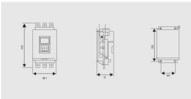
The External shape and installation dimensions of 75KW-560KW
