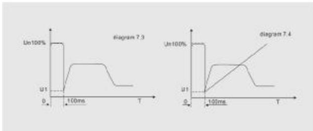
**Note:** This mode will cause big-current shock to the motor, so if the Ramp voltage or Limit-current mode can be used, please had better not use the Torque control to start
