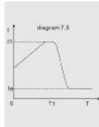
7.2.5 Double closed loop (Both Ramp Voltage and Limit-current)to start (The F9 items set as "5",this starting mode is in use) This starting mode uses the control mode of Ramp voltage starting and Limit-current starting Double Closed Loop circuit, it is a composite starting mode. The Output voltage waveform is changed as Motor and the load equipments.
